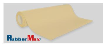
RM Biltrite® Rubbermax® Natural Rubber (NR) Grade 1 is manufactured using 100% treesourced latex to produce a low compression set, high tensile strength, superior resilience, and good abrasion resistance, tear resistance, and vibration dampening. Natural Rubber sheeting ingredients are FDA approved and can be used in the food or pharmaceutical industries. Not recommended for contact with hydrocarbons, ozone, UV, or strong acids.
